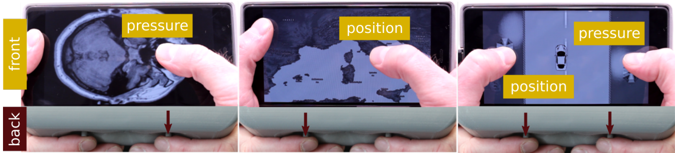
Fig. 13. Exemplary application scenarios for the proposed BoD force feedback approach: (top), a volume viewer, a racing game, a map viewer, all supported by force feedback on the back of the smartphone. For the Volume viewer, for example, the pressure on the touchscreen is directly translated to the pins' height. When mapping the position, the information at the point of contact is taken (e.g. elevation data) and transferred to the pin.
