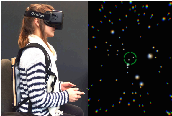
Figure 1: Experiment setup showing a participant in the upright (0°) condition wearing the HMD and backpack (left). Visual stimuli of the optic flow environment (right).
