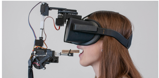
Figure 5. Adding biting functionality to FaceHaptics - showing the potential of extensibility, but also the limitations regarding reloading.
