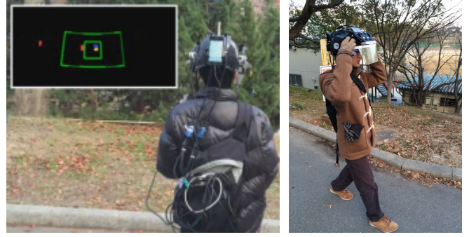
Fig. 6: The image projected onto the display, where black is transparent on the actual display (left), and a participant walking through the outdoor search task (right).
