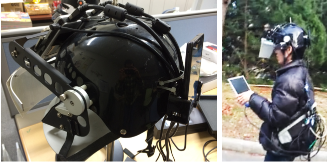
Fig. 3. Images showing a rear view of the OST display with the tracker used for outdoor label registration (left) and an outdoor test run of the device for the campus navigation task (right).
