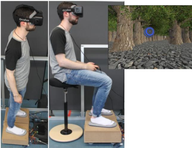
**Figure 3. User in standing leaning (left) and seated (middle) pose. Right: Test environment with follow-me object.**
