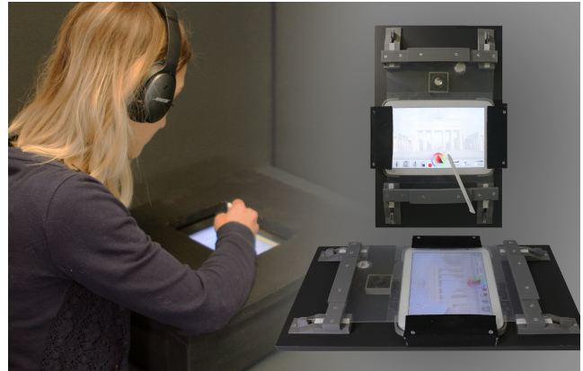
Figure 5. Apparatus with sound / visual cover (Left), top and side/top view of setup showing art application (Right).
