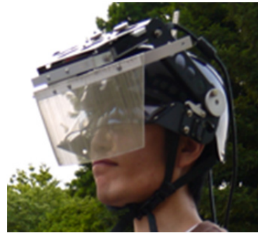
Figure 2: The wide FOV optical see-through HMD used in our experiments.
