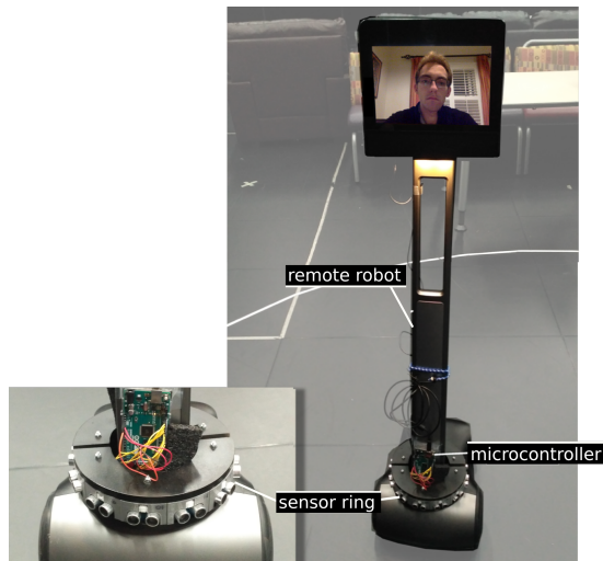
Figure 2: The ring consisting of 12 ultrasonic distance sensors attached to the Beam+ telepresence robot enables 360° coverage with a radius of up to 4m.
