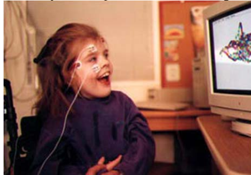
Figure 2.49: EagleEyes EOG-based eye tracking. Courtesy of Boston College
