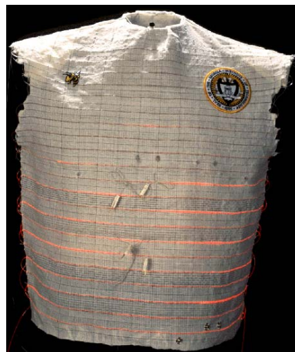
Figure 2.46: SmartShirt psycho-physiological monitoring garment. Courtesy of Georgia Tech / Sensatex
