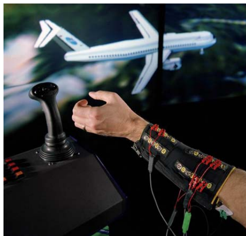
Figure 2.50: EMG-based control of an airplane Courtesy of NASA Ames Research Center
