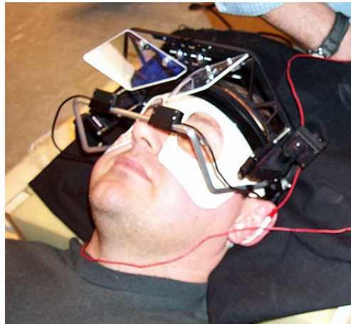
Figure 2.22: Galvanic vestibular stimulation interface. Courtesy of M. Jenkin
