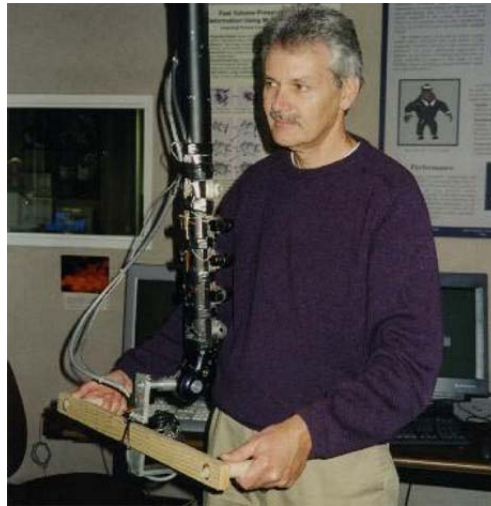
Figure 2.36: Collaborative stretcher carrying using haptics. Courtesy of R. Hubbold
