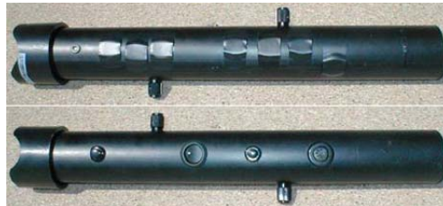
Figure 2.27: Pipe interface using wind pressure sensor. Courtesy of G. Scavone
