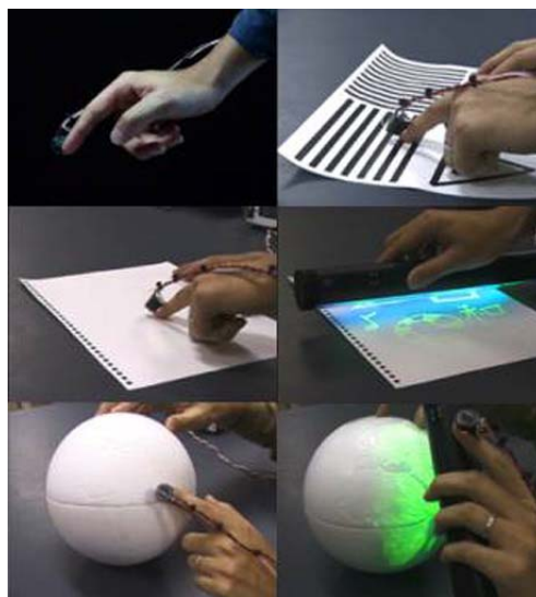
Figure 2.13: SmartFinger nail-mounted tactile device. Courtesy of JST & University of Tokyo
