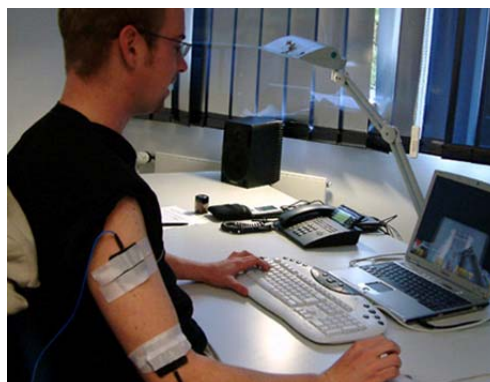
Figure 4.11: Test setup showing electro pads and display with Quake3.
